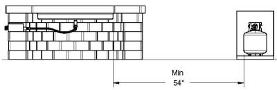
**WARNING:** Failure to follow location and mounting guidelines for the LP tank could result in serious injury.
