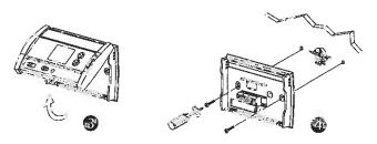
Gently tilt the thermostat upwards.
