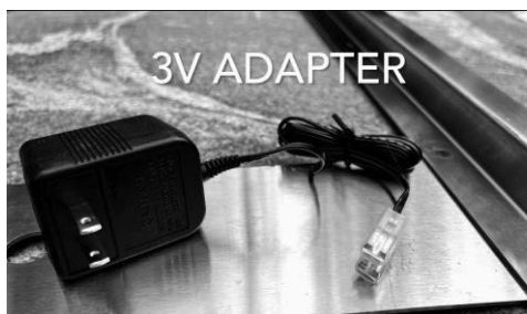
9- Either connect 3v adapter to module or use batteries.
