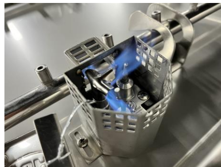
Figure 10.2 – Pilot flame coverage of thermocouple.
