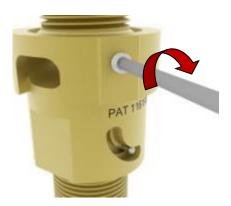
2. On the front side of orifice, use a #2 flat head screwdriver to rotate orifice from either NG to LP or LP to NG depending on proper gas type. Always ensure that the orifice insert, and collar are aligned.
