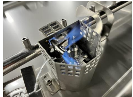
Figure 9.2 – Pilot flame coverage of thermocouple.
