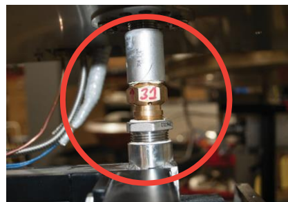
Figure 9.1 – Locating orifice for cleaning
