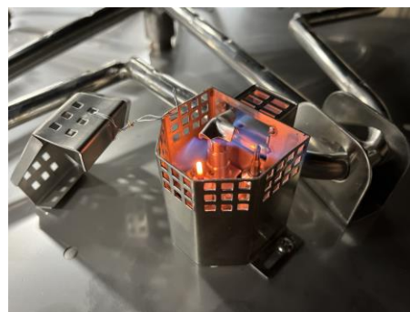
Figure 9.2 – Pilot flame coverage of thermocouple.
