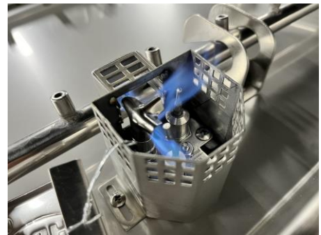
Figure 9.2 – Pilot flame coverage of thermocouple.
