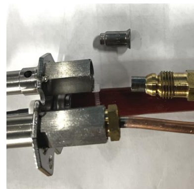
Figure 9.3 – Cleaning pilot orifice
