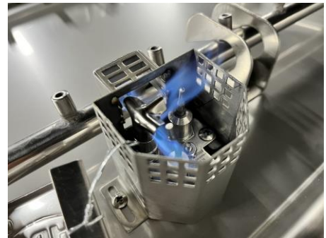
Figure 9.2 – Pilot flame coverage of thermocouple.
