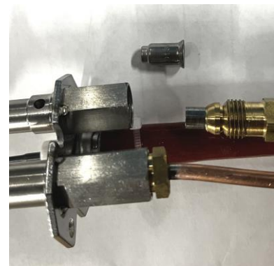
Figure 9.3 – Cleaning pilot orifice
