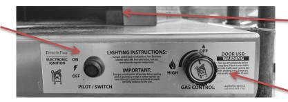
Pilot must be ignited for burner flame.
