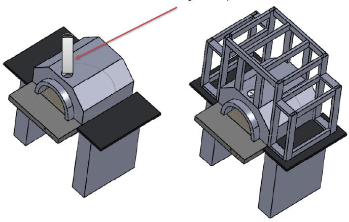
Oven built-in enclosure framing can either be constructed of steel studs **or concrete block**. Material used must be noncombustible.
