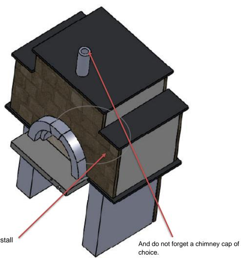
5- Once stone is installed, install desired roof material.
