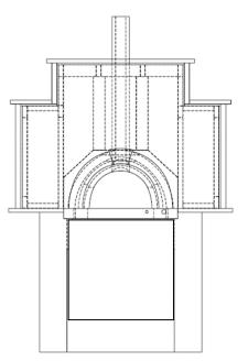
Unobstructed 12" overhang is necessary for accessing oven components and servicing.
