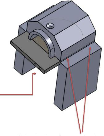
Bottom of oven must be kept unobstructed oven cannot be set on a continuous solid countertop.
