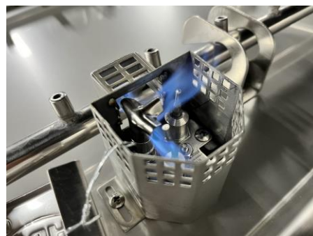
Figure 9.2 – Pilot flame coverage of thermocouple.
