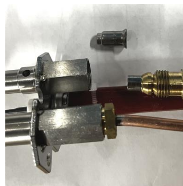
Figure 9.3 – Cleaning pilot orifice
